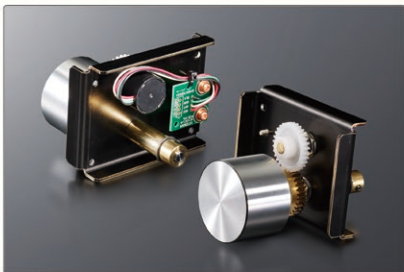
Rotary encoder and weighted rotation mechanism
